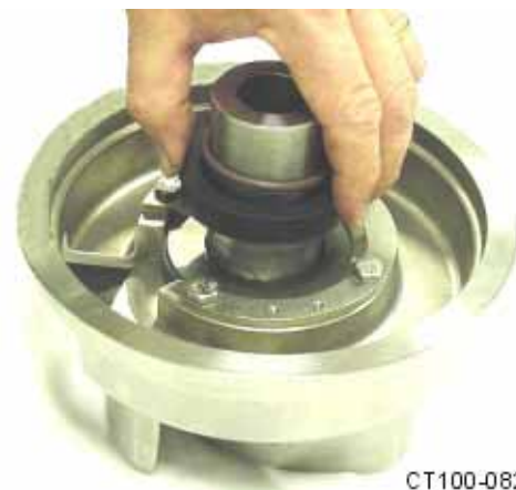
Figure 17 - Push Rotary Seal Down Until the O-ring is Released.
