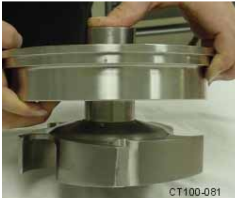
Figure 3 - Moving the Rotary Seal up the Shaft
