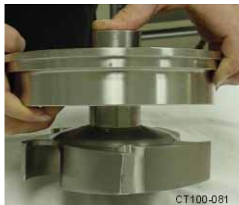
Figure 16 - Moving the Rotary Seal up the Shaft
